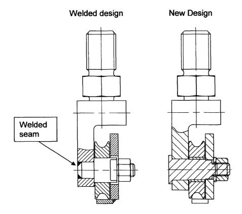
For the sake of good order, we have made additional tensile tests of the tool (welded design).
